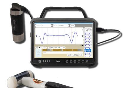
PET is used to test the integrity of deep pile foundations. PET Uses the pulse-echo method (PEM) for pile integrity testing (PIT).
