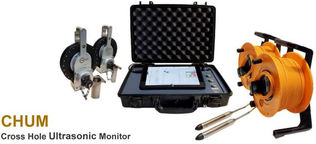
The CHUM (Cross Hole Ultrasonic Monitor) uses the Crosshole Sonic Logging CSL testing method to perform high-resolution quality control of deep foundations.
